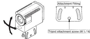
It is possible to angle the product by 45 degrees upward/downward or left/right if the provided attachment fittings are used. The two taps of the attachment fittings are the tripod attachment screws (W 1/4). By screwing the attachment fittings onto the main unit, the product can be attached to the tripod.
