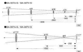
Note: The laser marker is aimed at the center of the measuring area
