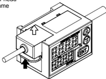
Amplifier has not a protective structure. When you connect the output cable and the sensor cable, make sure that the water or oil does not penetrate to the amplifier along the cable. When used in such an environment where water or oil might get in to the amplifier, please use optional protective case. (Equivalent to IP65)
