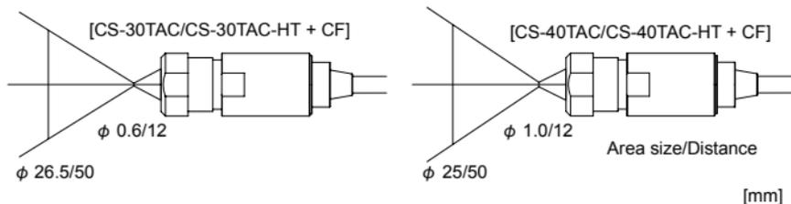
\* When the CF lens is attached, correction is necessary because light intensity received from the target decreases by 20 to 30%.
