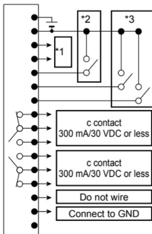
\*1 Connect to the 4-20 mA input of an analog device.
