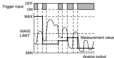
\* In the MAX HOLD, P-P HOLD and SAMPLE HOLD analog output remain the minimum value (4 mA) until the first trigger.
