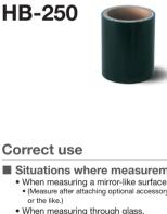
When attached to the surface of an object with unknown emissivity or a glossy object, this tape provides an emissivity of 0.95, enabling accurate non-contact temperature measurement. Emissivity on the PT-7LD can be switched between two levels. Set the emissivity to 0.95 (HOT) for use. The tape is built with material resistant to heat up to 250°C (482°F). Total area: 60 mm × 2000 mm
