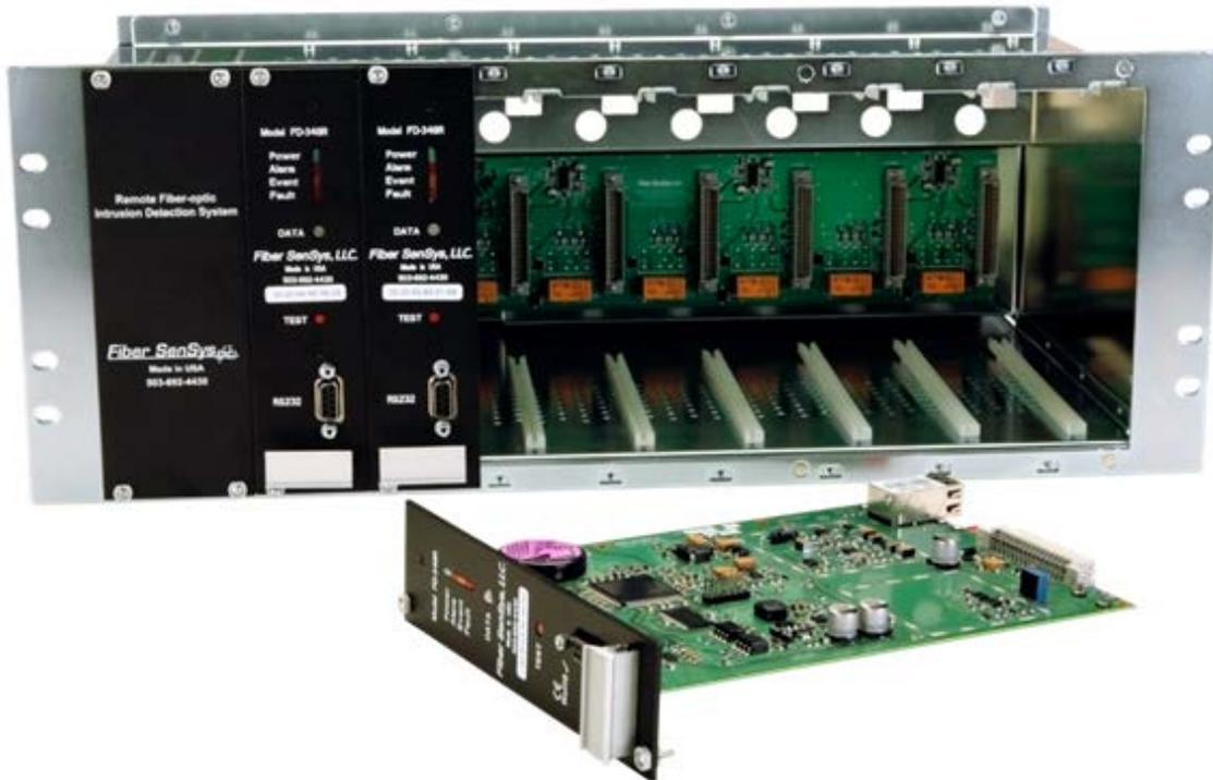
Figure 4-5. The RK348 with two installed FD348R APU modules and another APU in front
