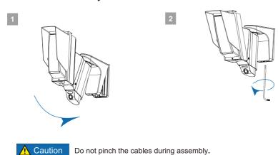
Do not pinch the cables during assembly.
