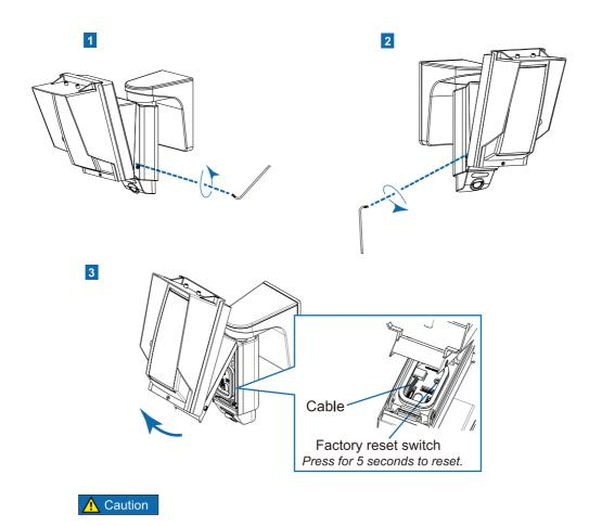
Do not pinch the cables during assembly.
